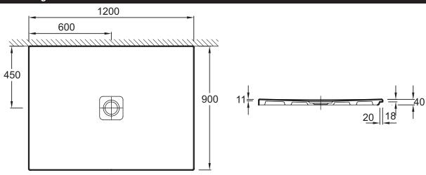
Product Specification: Extra-slim rectangular ceramic shower tray 120 x 90 x 4 cm. N147K. Collection: REPLAY. Dimensions: 120 x 90 x 4. Weight: 39 kg. Material: Ceramic. Installation: Floor-standing or inset. Shape: Rectangular. Shape: Rectangular. Shape: Rectangular. Floorstanding or inset. Anti-slip glaze. Order with special drain and cover 9276K. Waste Ø 90 mm.
