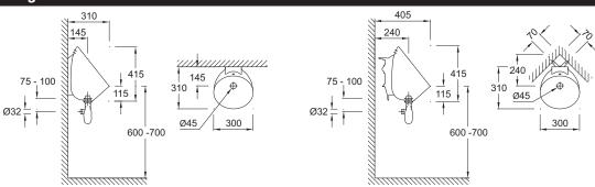
Product Specification: Urinal with water effect. E1519. Collection: HORS COLLECTION. Dimensions: 31 x 41.5. Weight: 7.6 kg. Material: Ceramic. Installation: Wall-mount.
