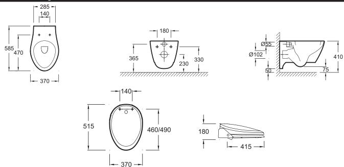
Product Specification: Wall-hung WC pan with multifunctional bidet seat. C45559K. Collection: PRESQU'ILE AND VIA. Dimensions: 58.5 x 37 cm. Weight: 31.4 kg. Material: Ceramic. Installation: Wall-hung. Wall-hung WC pan 45534CK included, adapted to fit with bidet seats. Bidet seat C3-225 included. Remote control. 2 nozzles (rear and front) with oscillating movement. Auto clean nozzle before and after use Adjustable water temperature and pressure. Air drier. Heated seat. Auto open / close seat.
