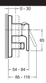
Product Specification: Trim and lever for built-in bath-shower mixer. 98720D. Collection: MODULO. Installation: Built-in. Flow rate: 30 I/min / 25 I/min. Incl. single-lever built-in mixer. Incl. non-return valve. Automatic diverter with locking option. Ceramic disk cartridge. DVGW NW-6512CP0428.
