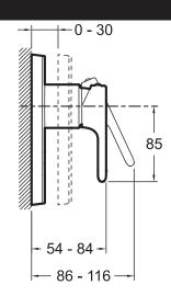
Product Specification: Trim and lever for built-in shower mixer. 98708D. Collection: MODULO. Weight: 1.9 kg. Installation: Built-in. Normes: ACS (Certificate of Sanitary Compliance): 10 ACC LY 004. Flow rate: 40 l/min. Incl. single-lever built-in mixer. Incl. non-return valve. Ceramic disk cartridge. DVGW NW-6512CP0427.
