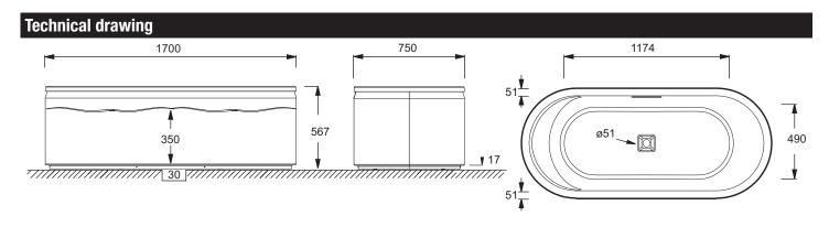
Product Specification: Cast iron bath, freestanding, 170 x 75 cm. 9287. Collection: LOVEE. Dimensions: 170 x 75. Weight: 132 kg. Material: Cast iron. Installation: Countertop. Volume: 231. Shape: Rectangular. Anti-slip coating.
