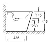
Product Specification: Back-to-wall floor-standing bidet. 5040K. Collection: RÊVE. Dimensions: 56 x 36.5. Weight: 29.5 kg. Material: Ceramic. Installation: Floor-standing. Faucet drilling: 1 faucet hole. Fixings: Concealed floor fixings included. Bidet with contemporary lines. Slow-close cover E4818 and metal hinges included. Chromed overflow cap.
