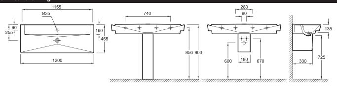
Product Specification: 1-hole vanity top 120 cm. 5025K. Collection: REVE. Dimensions: 120 x 46.5. Weight: 38.6 kg. Material: Ceramic. Installation: Self-supporting. Can be mounted onto specific cabinet. with or without pedestal/semi-pedestal/semi-pedestal/shroud. Faucet drilling: 1 central faucet hole. Wide ledge for optimal comfort of use. Combination of straight lines and softened angles. Perfect fit with cabinet. With 3 tap holes 5025K-8.
