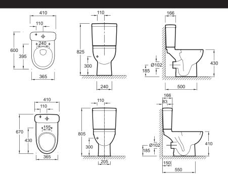
Product Specification: Cistern. 18581W. Collection: REACH. Weight: 13.5 kg. Material: Ceramic. Water-saving button 3/6 L. Inlet bottom left.
