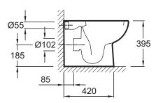
Product Specification: Back-to-wall pan. 18154W. Collection: PANACHE. Dimensions: 55 x 35.8. Material: Ceramic. Vario outlet. Standard or slow close seat and metal hinges. 2-volume flow technique 3/6 l.
