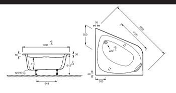
Product Specification: Corner bath 140 x 140 cm. 15563K. Collection: REACH. Dimensions: 140 x 140. Weight: 29 kg. Material: Acrylic. Installation: Built-in. Volume: 250/180. Shape: Corner. Corner solution for a space-saving concept.. Ergonomic shape for optimal bathing comfort.. Black pillow included.. Tap deck and waste at foot end for easy access and maintenance.. Wide ledge can accommodate a bathscreen.. Fast assembly with Quick Clip foot system..
